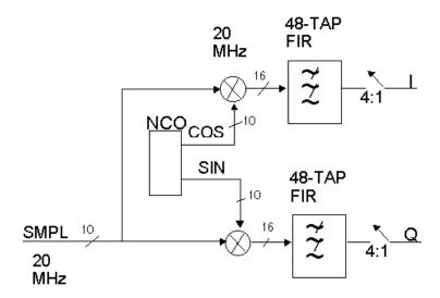
This demodulator consists of a channel demodulated with a Sine and Cosine function.
