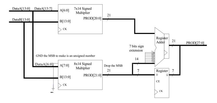
**Upper Half Multiplier**: Used to multiply the upper half of DataA time DataB. Both DataA and DataB's MSB represent the sign bit in this case so the multiplier to generate is a 7x14 Signed multiplier.
