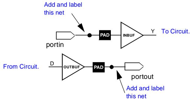
Figure 3-1. I/O Pins in a Mentor Graphics Design
